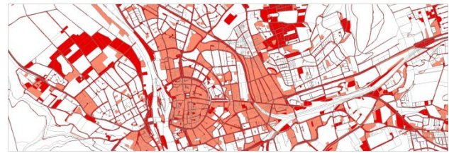
Figure 3: Comparison of the land-use in the cadastral and topographic dataset: Objects of different land-use domains are displayed in dark red, with same domain in light red and with identical classes in white.
