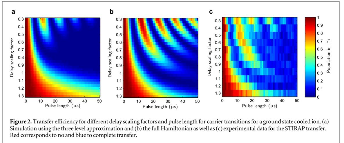
**Figure 2.** Transfer efficiency for different delay scaling factors and pulse length for carrier transitions for a ground state cooled ion. (a) Simulation using the three level approximation and (b) the full Hamiltonian as well as (c) experimental data for the STIRAP transfer. Red corresponds to no and blue to complete transfer.
