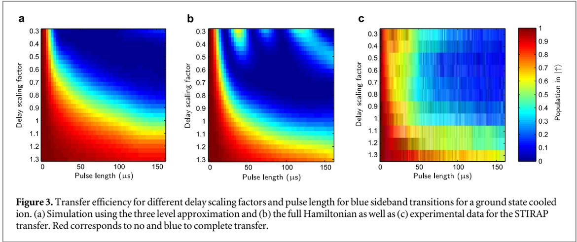
**Figure 3.** Transfer efficiency for different delay scaling factors and pulse length for blue sideband transitions for a ground state cooled ion. (a) Simulation using the three level approximation and (b) the full Hamiltonian as well as (c) experimental data for the STIRAP transfer. Red corresponds to no and blue to complete transfer.
