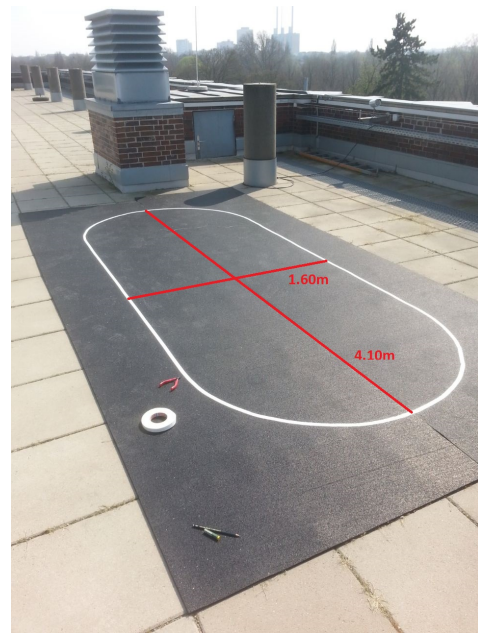
Fig. 4. Trajectory used in the experiment: dark rubber mats with white contrast tape for the optical trace sensor.
