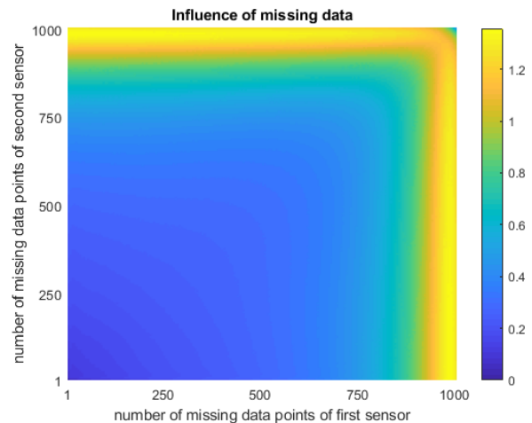
Fig. 7. Influence of missing data for two sensors
