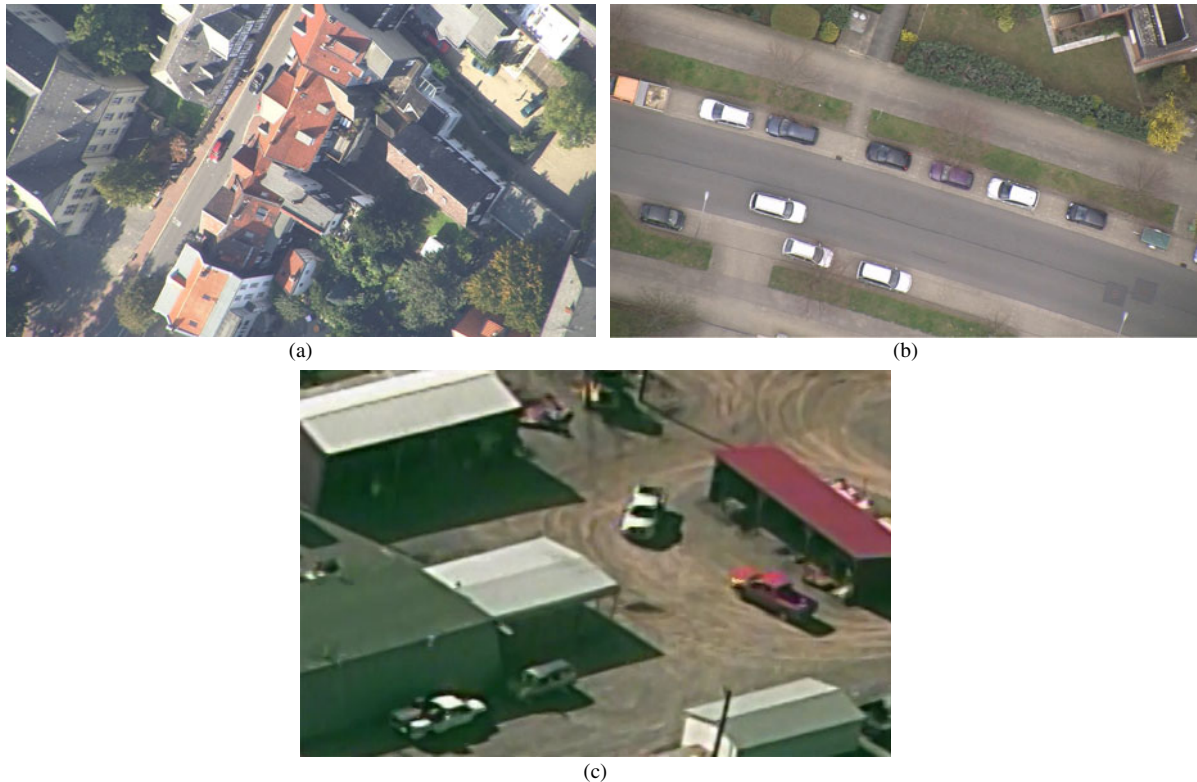
Fig. 7. Example frames of the test set used to evaluate the MO detection and ROI coding framework. ( Test Set 1 ). (a) MOs (black and red car with shadows) in the 750 m sequence, HDTV resolution, ground resolution: 21 pel/m [34, 39]. (b) MO (white car in the middle) in the 350 m sequence, HDTV resolution, ground resolution: 43 pel/m [34, 39]. (c) MOs (white and red car in the middle) in the VIRAT test data set, original resolution: 720 \times 480 , interlaced [37, 38].
