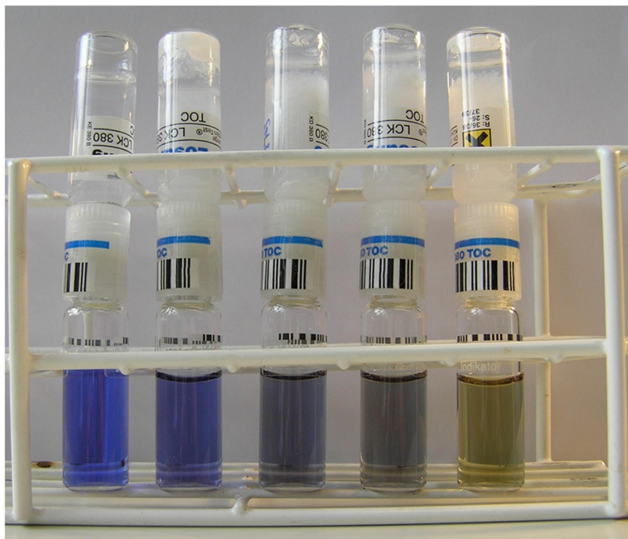
Figure 2 Color change of indicator cuvettes due to the amount of TOC in the sample. Cuvettes show zero, 10, 25, 35, 50 ppm TOC, respectively (from left to right).
