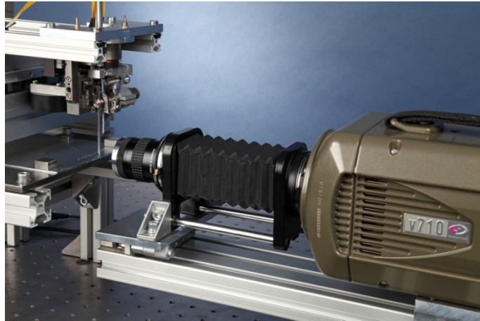
Fig. 4.4: High-speed observation system
