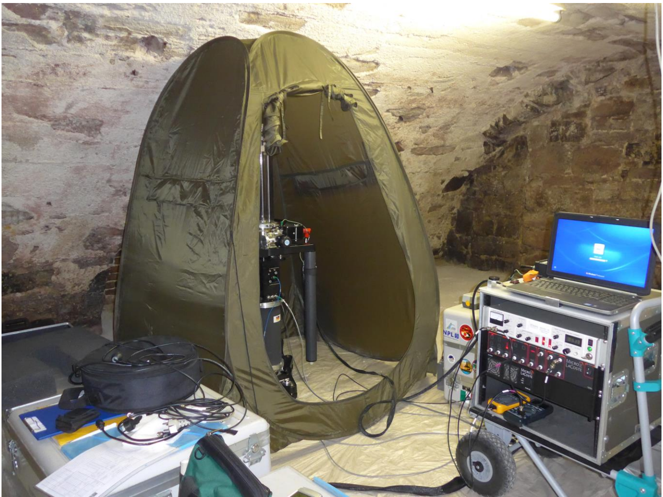
Figure 2: The situation for the absolute gravimeter FG5X-220 in the town hall (cellar vault), August 2018. The point is officially marked and documented by the “Landesamt für Vermessungswesen und Geoinformation” of Thuringia. To avoid dirt falling down from the ceiling, a cover tent was deployed.
