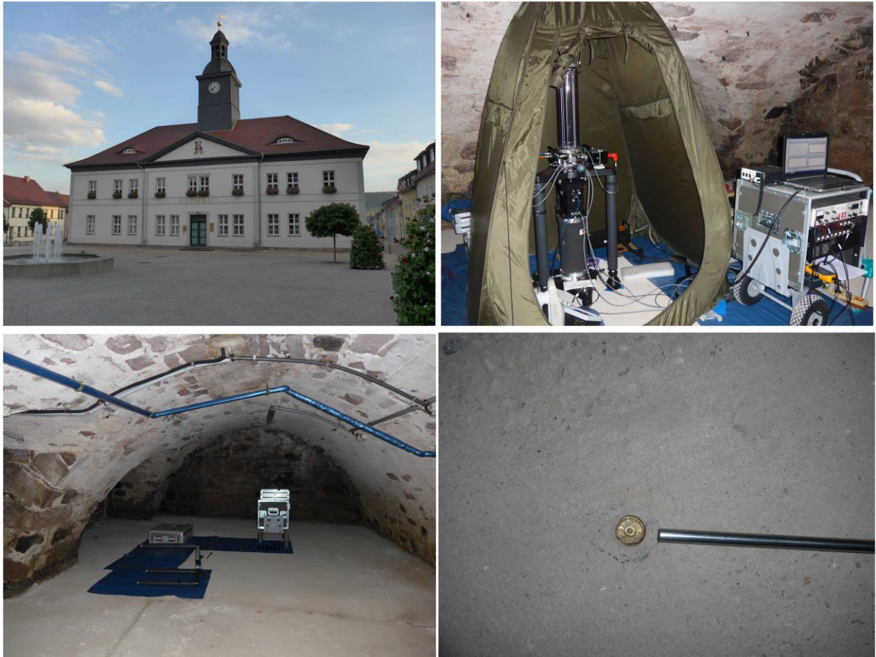
Figure 2: The situation for the absolute gravimeter FG5X-220 in the town hall (cellar vault), August 2016. The point is officially marked and documented by the “Landesamt für Vermessungswesen und Geoinformation” of Thuringia. To avoid dirt falling down from the ceiling and to solve the humidity issue with a small heater, a cover tent was deployed.
