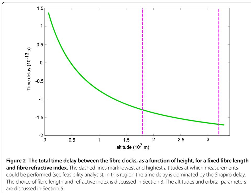
low satellite altitudes the time delay is positive and dominated by the special relativistic dilation, whereas at high altitudes it is negative and dominated by the general relativistic dilation. Therefore care must be taken to launch the satellite into a sufficiently high orbit for the general relativistic time dilation to be the dominant effect. Figure 2 demonstrates that the Shapiro delay for a satellite at the orbital heights considered in this proposal is of the order 100 fs.
