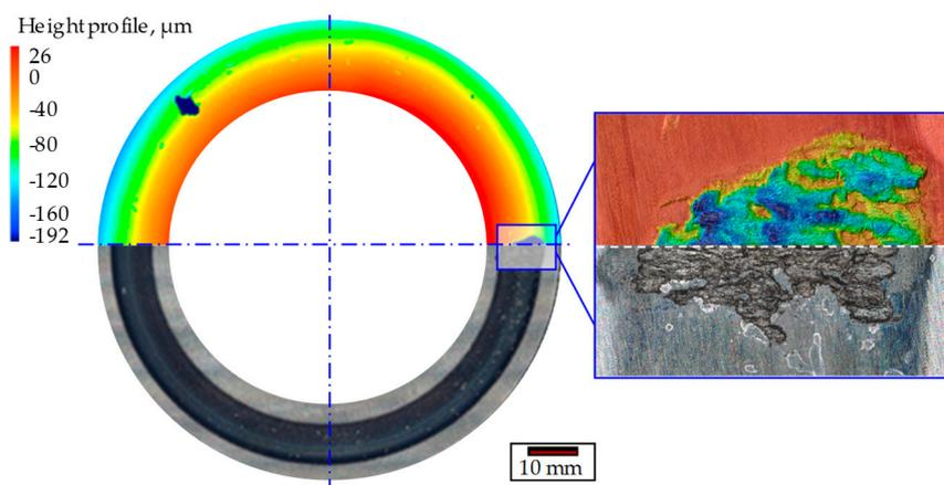
**Figure 12.** Tailored forming bearing washer after rolling contact load test (running time of 332 h).
