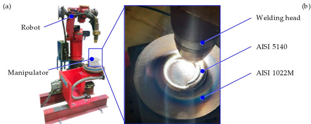
**Figure 2.** Experimental setup of PTA welding (a), PTA-process (b).
