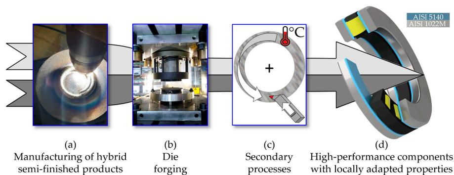
**Figure 1.** Process chain for manufacturing a hybrid axial bearing washer by tailored forming. (a) Plasma-transferred arc deposition welding, (b) hot forming, (c) mechanical processing and heat treatment, (d) Bearing assembly for use in a test bench.
