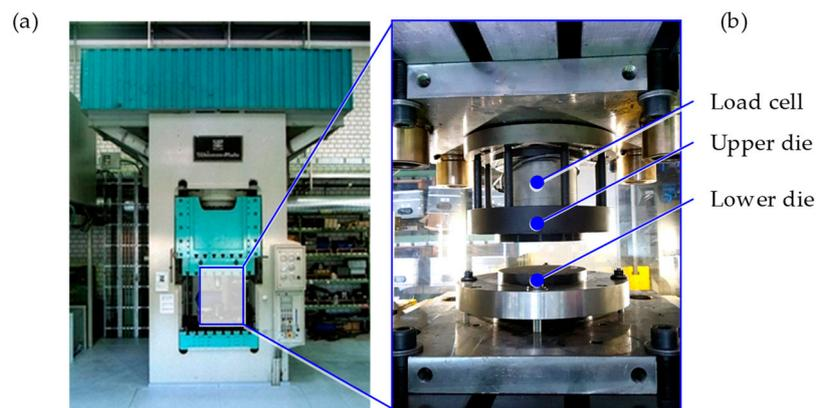
**Figure 4.** Hydraulic forming press (a), forming tool system for forging of the bearing washers (b).
