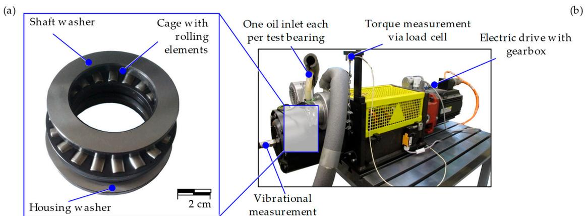
**Figure 10.** Assembled bearing consisting of tailored forming bearing washers, cage, and rollers (a); FE8 rig for investigation of fatigue of two tailored forming bearings simultaneously (four washers per test, (b).
