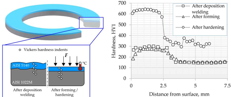
**Figure 7.** Hardness gradients of the hybrid bearing washers.
