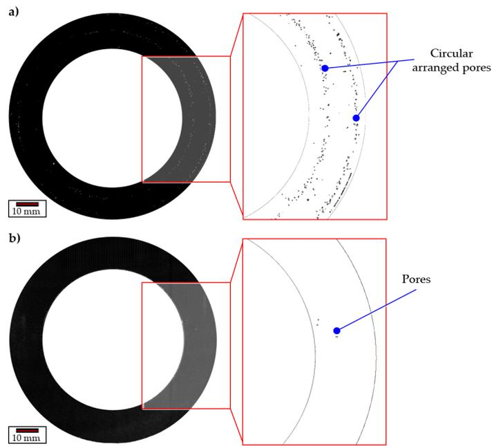
**Figure 9.** Scanning ultrasonic microscopy of a tailored forming bearing washer: (a) after joining and before forging, showing subsurface pores aside the welding lines (indicated as white spots), (b) after forging, showing a reduction of subsurface pores (indicated as white spots); zoom images edited by inverting the color range.
