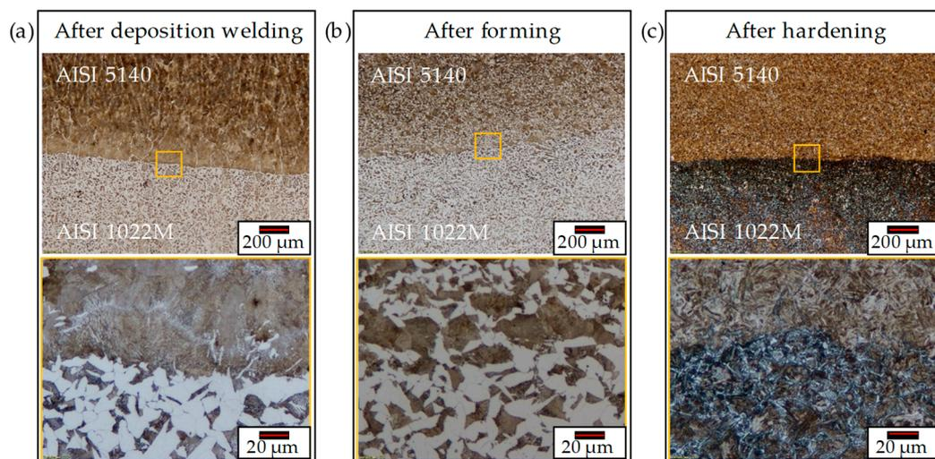
**Figure 6.** Micrograph of the joining zone after deposition welding (a), after forging (b) and after hardening (c).
