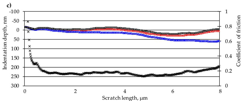
**Figure 8.** Results of the scratch tests: (a) industrial bearing washer made of conventional rolling bearing steel AISI 52100; (b) hybrid bearing washer without additional deformation; (c) hybrid bearing washer with additional deformation.
