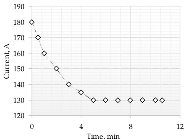
Figure 3. Current intensity curve during cladding process.
