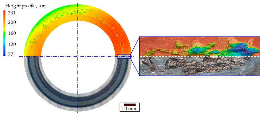
**Figure 11.** Bearing washers which were not forged after the cladding process after rolling contact load test (running time of 237 h).
