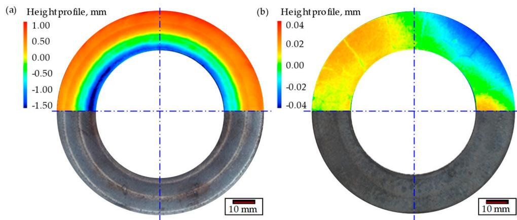
**Figure 5.** Height profile of the hard-faced area before (a) and after forging (b).
