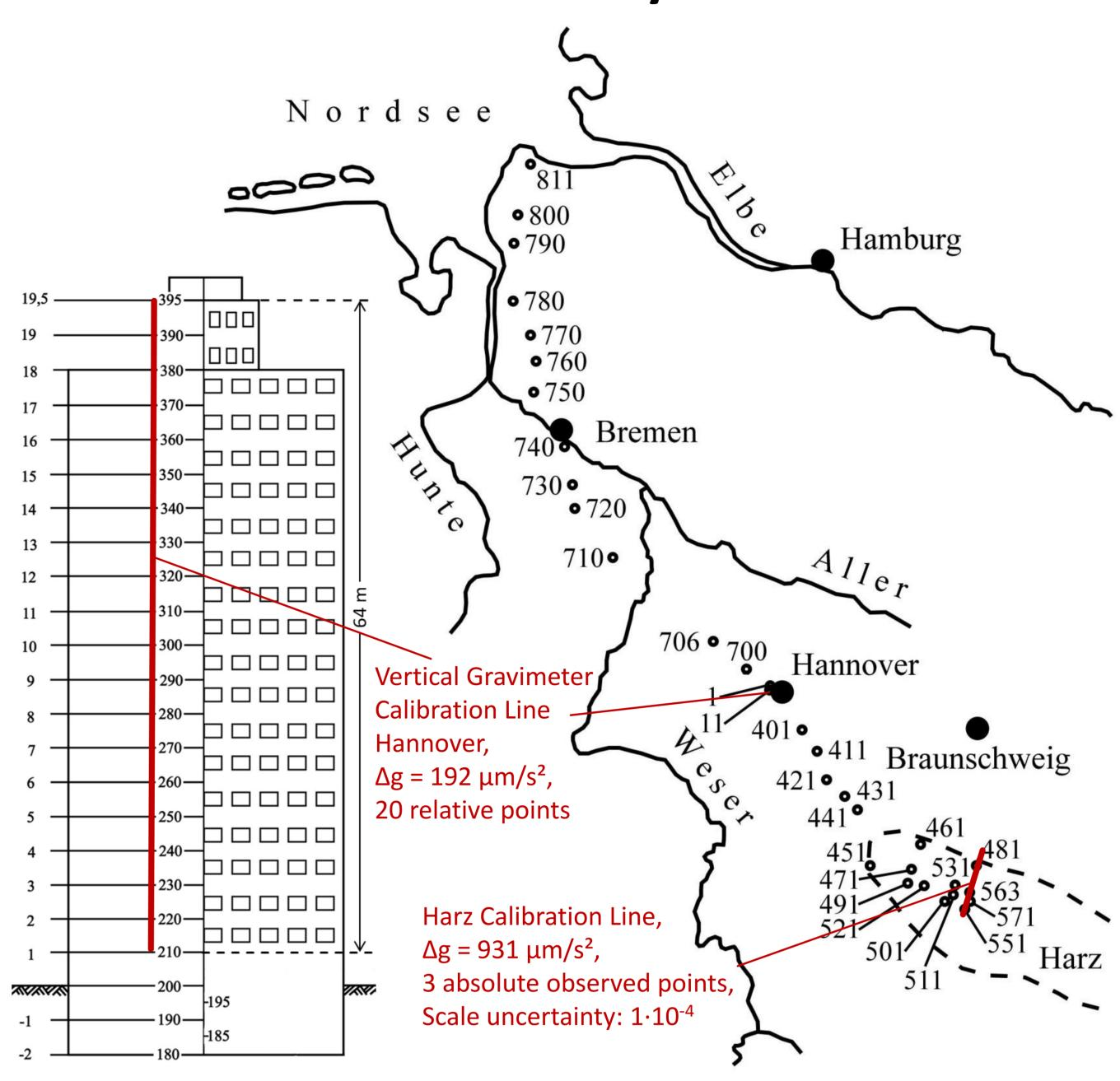
The Gravimeter Calibration System Hannover with its two most important parts (in "red"):
