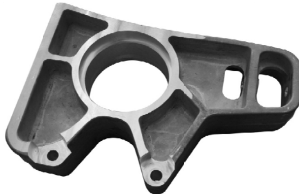
Figure 8. Load-sensitive magnesium wheel carrier from the RP09 race car (Team Horsepower, Leibniz Universität Hannover).
