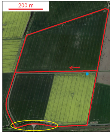
Figure 4.2: Test track of kinematic car experiment: the yellow ellipse depicts a natural alley with signal obstructions, the blue dot indicates the location of the local reference station, the red arrow indicates starting point and driving direction of each eight-shaped test drive (source of map: Google Maps)
