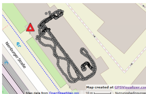
Figure 4.25: Trajectory of the pedestrian experiment, where the reference station is indicated by a red triangle
