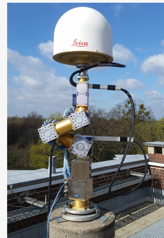
Figure 1: IfE robot for absolute antenna calibration.
