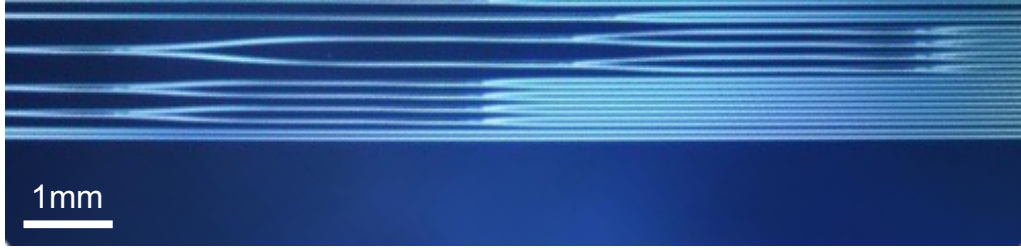
Figure 7.1: Micrograph of beam splitter structures on the used silicon hot embossing stamp [44].
