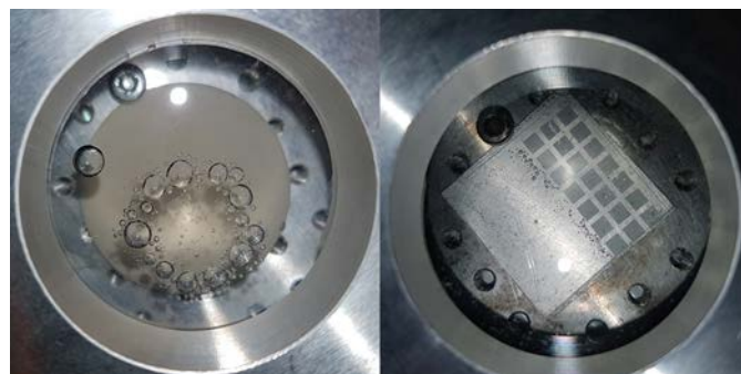
Fig. 1. (left) bubble accumulation with pump switched off; (right) no bubbles with pump switched on. The free diameter of the entrance window is 40mm.
