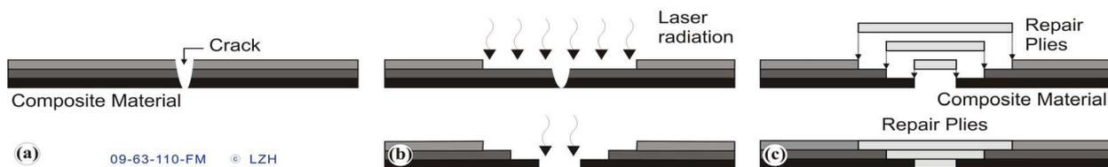
Figure 1. Principle of laser-based preparation for bonded repair of composite materials. (a) cracked CFRP specimen; (b) laser-based ply-by-ply removal; (c) refilling and consolidation with (e.g. laser-cut) fiber plies.
