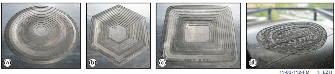
Figure 7. (a)-(c) Various geometries for bonded repair; (d) Laser machined step structure on curved surface.
