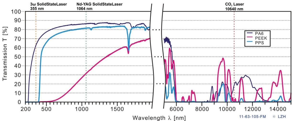
Figure 2. Transmission characteristic of selected thermoplastic matrix materials with indication of relevant laser wavelengths.
