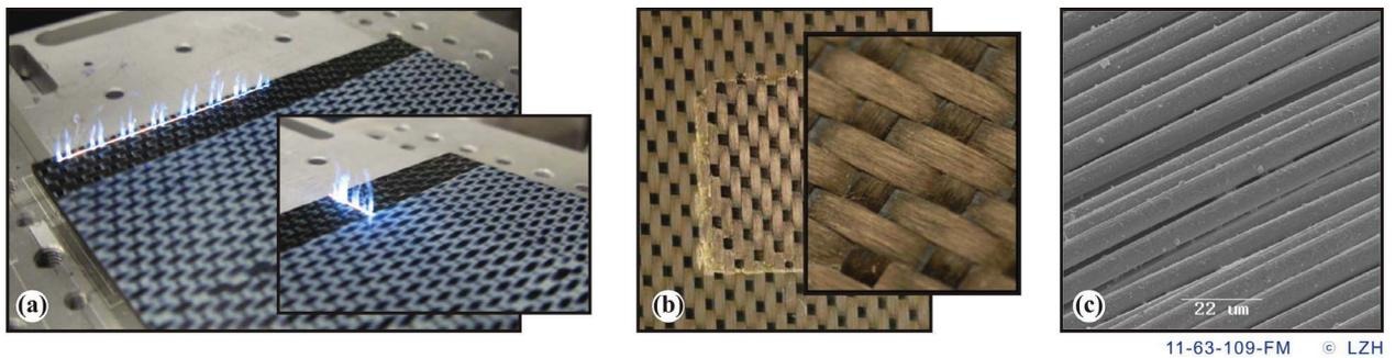
Figure 5. Selective ablation of the matrix material without damaging the fibers: (a) areal ablation principle (in x- and y-direction); (b) partly removed matrix from fabric; (c) SEM picture of cleanly exposed and non-damaged carbon fibers.
