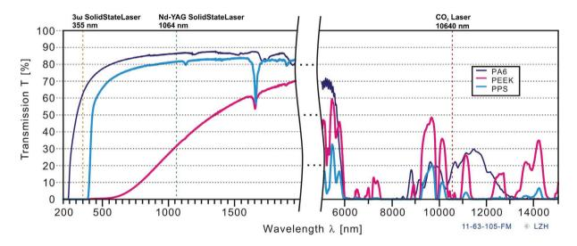
Figure 2. Transmission characteristic of selected thermoplastic matrix materials with indication of relevant laser wavelengths.
