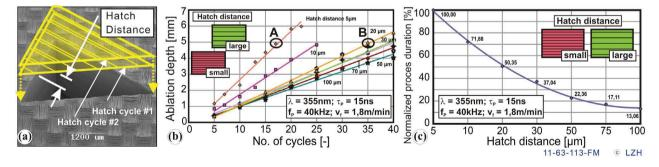
Figure 4. Influence of hatch distance and number of cycles of the affective ablation depth: (a) definition of hatch distance and number of cycles; (b) influence of hatch distance on the ablation depth; (c) potentials for increased throughput in dependence on hatch distance.
