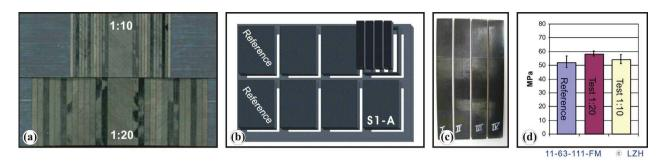
Fig. 6. Bonded repair: (a) size of area with different step width; (b) test pattern according to DIN 65148; (c) separated test specimen; (d) results of shear strength tests in comparison to non-machined specimen (reference).
