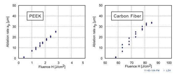
Figure 3. Ablation rate of the matrix material PEEK and carbon fibers vs. fluence (wavelength  $\lambda = 355$ nm; pulse duration  $\tau_p = 30$ ns) [3].
