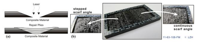
Figure 8. (a) Principle for bonded repair with continuous scarf angle; (b) laser-machined part for demonstration of a continuous scarf angle.
