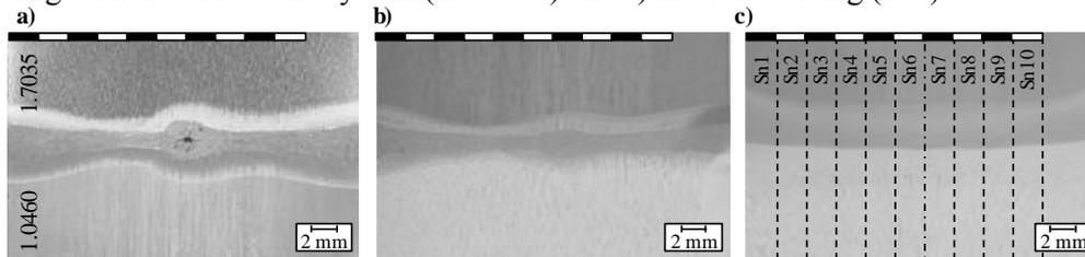
**Figure 3.** Longitudinal grinding of hybrid semi-finished products according to: a) LWwoUS; b) LWwUS; c) FW
