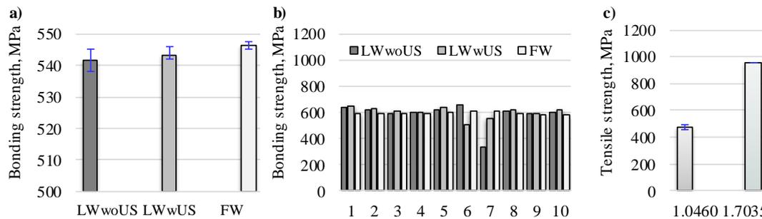
**Figure 5.** a) Determination of the global bond strengths; b) The bond strengths of the hybrid semi-finished products; c) tensile strengths of the mono materials according to the literature [8]
