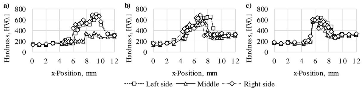
**Figure 4.** Hardness gradients of the hybrid semi-finished products: a) LWwoUS ; b) LWwUS; c) FW
