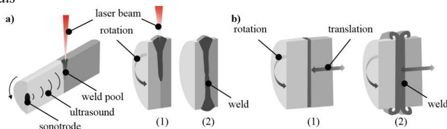
**Figure 1.** Schematic drawing of the specimen geometries in cross section during (1) and after (2) welding: a) laser beam welding; b) friction welding
