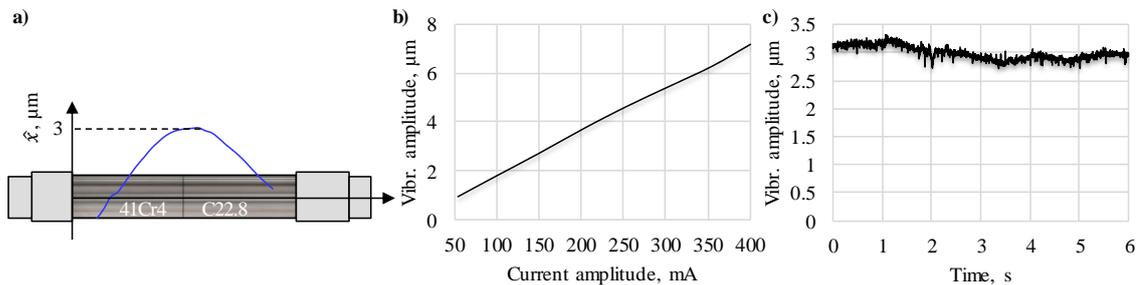
**Figure 2.** a) Measured vibration distribution along the workpieces b) dependency between vibration amplitude and measured current amplitude at measurement converter c) measured vibration amplitude during welding process
