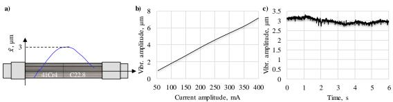
Figure 2. a) Measured vibration distribution along the workpieces b) dependency between vibration amplitude and measured current amplitude at measurement converter c) measured vibration amplitude during welding process
