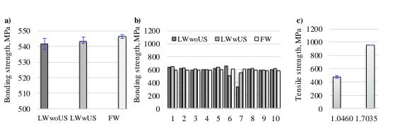
**Figure 5.** a) Determination of the global bond strengths; b) The bond strengths of the hybrid semi-finished products; c) tensile strengths of the mono materials according to the literature [8]
