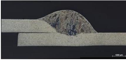
Fig. 3. Microsection of a laser stabilized reference weld with  $P_L = 340$  W,  $v_s = 0.6$  m/min,  $U = 16.2$  V,  $v_D = 2.3$  m/min.
