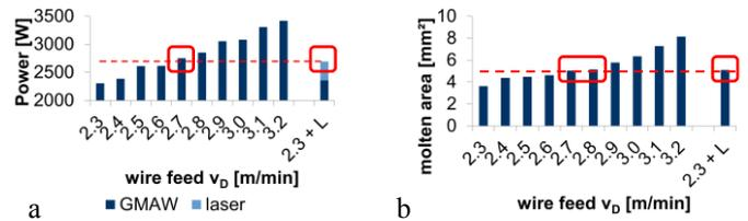
Fig. 5. (a) Measured power and (b) molten area of the compared processes relative to the wire feed.
