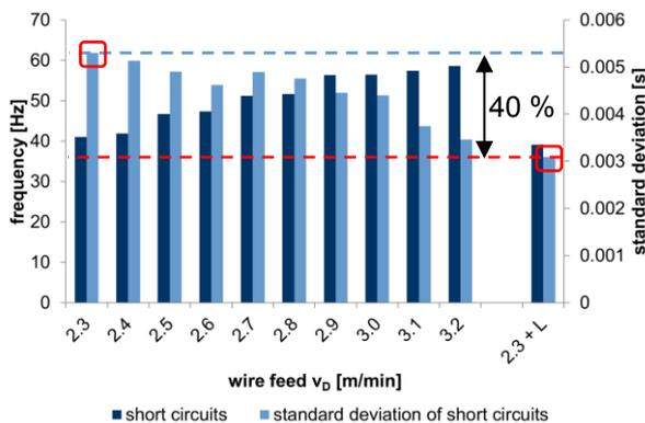
Fig. 7. Frequency of short circuits and standard deviation of their temporal occurrence.
