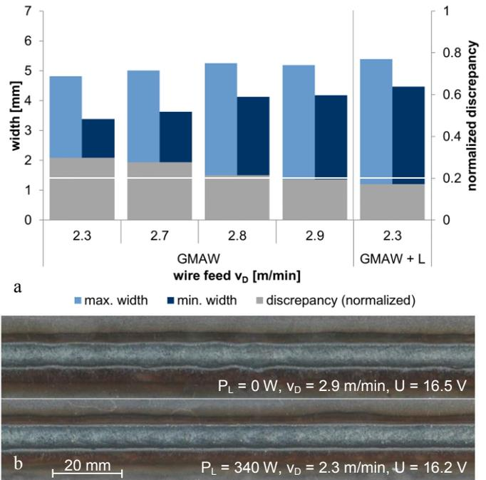
Fig. 8. (a) Maximum and minimum width on the top surface with normalized discrepancy of selected parameters; (b) top of exemplary GMAW and laser stabilized welds.
