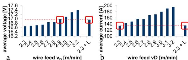
Fig. 4. Measured and averaged (a) voltage and (b) current of the used parameters, red line marks parameter with laser stabilization.
