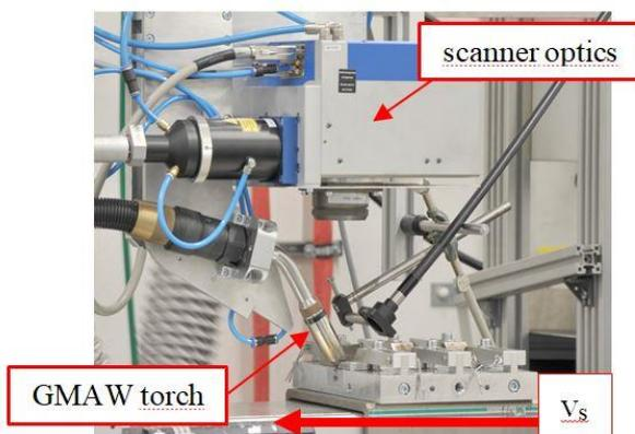
Fig. 1. Setup with 2 inch scanner optics. Neutral laser position, GMAW torch angled, welding direction marked with  $v_s$
