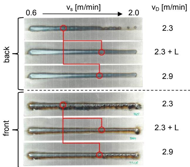
Fig. 9. Ramped weld speed  $v_s = 0.6$  to  $2.0$  m/min applied on GMAW with the start parameter  $v_D = 2.3$  m/min, the laser stabilized process and GMAW with raised energy. Red circles mark characteristics on the back sides of the samples and are transferred to the front sides.
