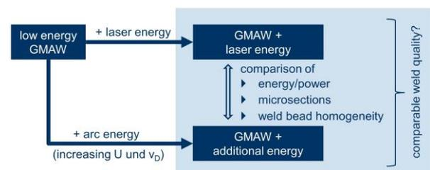
Fig. 2. Methodology for comparing the laser stabilized process with normal GMAW.
