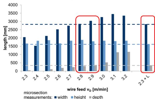
Fig. 6. Microsection measurements: width, height and depths of the weld beads, with dashed lines at the laser stabilized values
