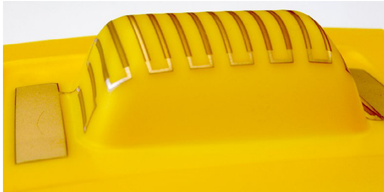
Figure 1: Deep drawn polystyrene sheet. The substrate is metallized and laser fine structured.
