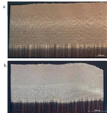
Fig. 3: SX-cladding without (a) and with (b) preheating
