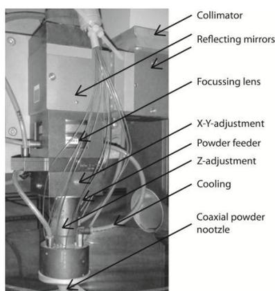
Fig. 5: Optical components and coaxial powder nozzle
