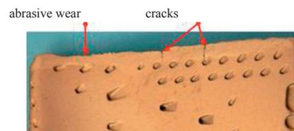
Fig. 4: Damage on turbine blade tip
