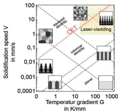
Fig. 2: CET - columnar to equiaxed transition [2]
