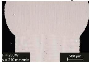
Fig. 7: Microscopic picture of the cross section of laser clad CMSX-4 with large volume (multi-track layer)
