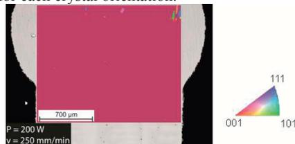
Fig. 8: EBSD analysis of CMSX-4 clad
