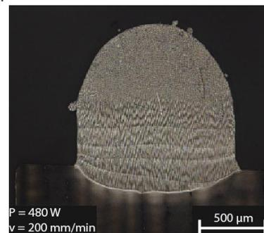
Fig. 6: Cross section of laser clad CMSX-4 sample (single-track per layer)
