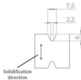
Fig. 9: Notch geometry
