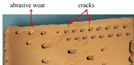
Fig. 2. Damage on turbine blade tip.
