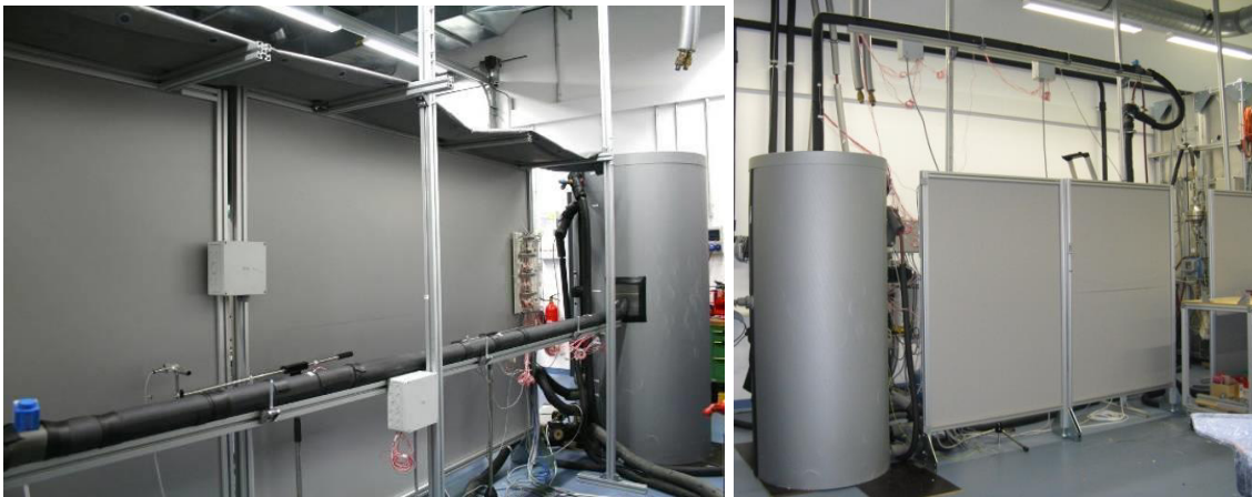
Fig. 2: Left: Test facility with improvements like the the continuous aluminium profile for exact adjustment of the test pipe (correct to 0.1^\circ ); Right: Test facility with a combination of a vertical and a horizontal pipe segment connected to the storage connector on top. The picture shows test pipe setup (B) according to chapter 3.5.
