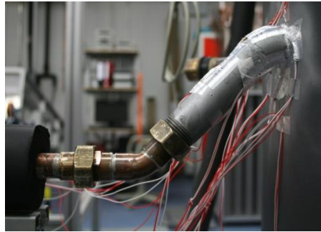
Fig. 8: Sloped storage connector in detail
