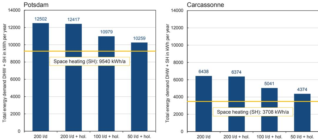
Fig. 3 Total energy requirement of the simulated system variants, split into space heating (SH) and domestic hot water portion (DHW) by the yellow line, for different average daily tapping volumes between 50 and 200 l/d, and the inclusion of a 2-week holiday period (" + hol.") from 25<sup>th</sup> July to 7<sup>th</sup> August without DHW-tapping; left for the site of Potsdam, right for the location Carcassonne.
