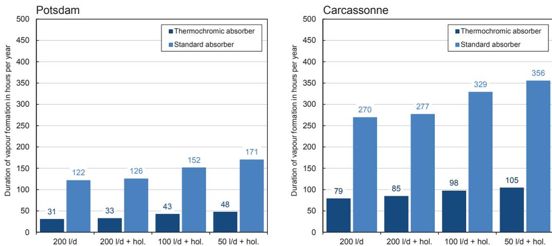
Fig. 6 Cumulated time in hours per year, in which evaporation in the solar circuit can occur (“duration of vapour formation”) for different average daily DHW tapping volumes between 50 and 200 l/d and the inclusion of a 2-week holiday period (“+ hol.”) from 25<sup>th</sup> July to 7<sup>th</sup> August without any tapping; left for the site of Potsdam, right for the location Carcassonne.
