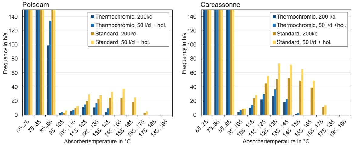
Fig. 5 Frequency distribution of the absorber temperature respectively for the lowest (50 l/d + hol) and the highest DHW demand (200 l/d) of the studied variations with the thermochromic absorber and the standard absorber; left for the site of Potsdam, right for the location Carcassonne.
