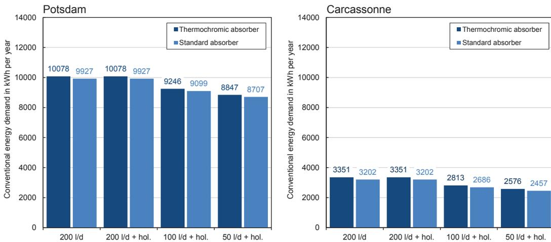
Fig. 4 Conventional energy provided by the gas boiler in kWh/a for different average daily tapping volumes between 50 and 200 l/d, and the inclusion of a 2-week holiday period (" + hol.") from 25<sup>th</sup> July to 7<sup>th</sup> August without DHW-tapping; left for the site of Potsdam, right for the location Carcassonne.
