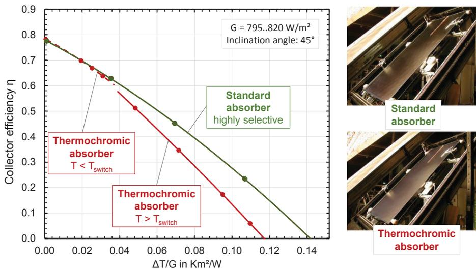
Fig. 2 Measured efficiency characteristics of the new flat plate collector prototype with a thermochromic absorber at temperatures below and above the switching temperature, compared to an identical collector with a common highly selective absorber coating.
