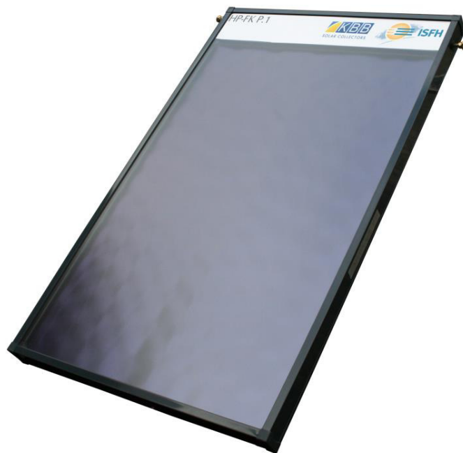
Fig. 6. Flat plate collector prototype with aluminum heat pipes. The solar circuit fluid only flows through the manifold, which is located at the top of the collector and is not part of the absorbing surface. Standard flat plate collector framing, transmittance of glass cover: \sim 90\% , absorptance of absorber: \sim 95\% , thickness of backside insulation: 50 mm
