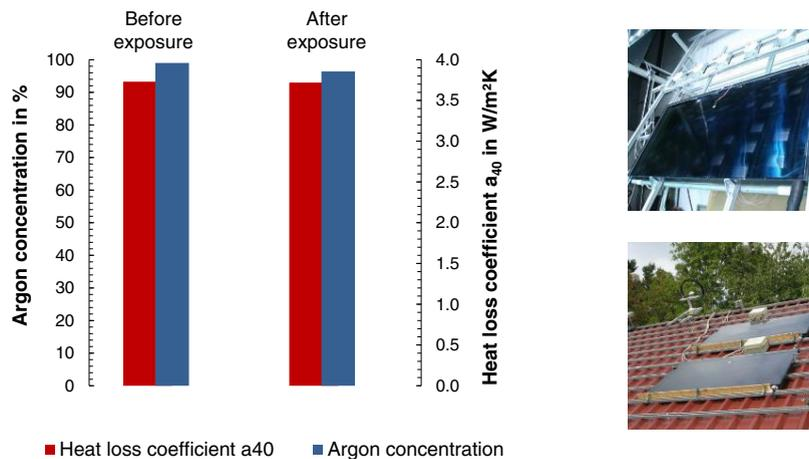
Fig. 8. Change in heat loss coefficient  $a_{40}$  and argon concentration of selected glass collector prototypes after shock-tests in our sun simulator (left) and exposure tests running at ISFH (right)
