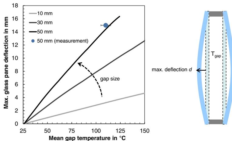
Fig. 7. Maximum deflection of a 1 x 2 m<sup>2</sup> large and 4 mm thick glass pane in an argon-filled double glazed unit at 90° tilt angle in dependency of the mean temperature of the gap: calculation according to [14] as well as single point indoor measurement on a triple-glazed collector prototype under stagnation conditions ( $G = 970 \text{ W/m}^2$ ,  $T_a = 30^\circ\text{C}$ , no wind)
