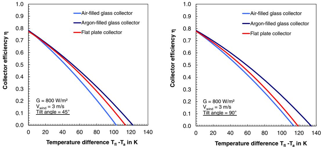
Fig. 5. Measured collector efficiency curves of air- and argon-filled triple-glazed prototypes, with an overall thickness of 60 and 50 mm respectively, at 45° (left) and 90° (right) tilt angle compared to those of a common flat plate collector
