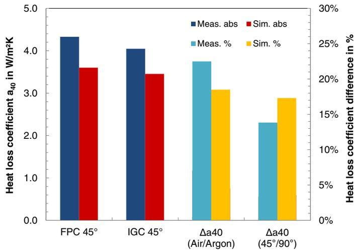
Fig. 6. Comparison of measured and simulated effective heat loss coefficients  $a_{40}$  of triple-glazed glass collectors and a common flat plate design
