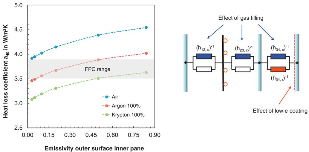
Fig. 3. Calculated “center-of-glass” heat loss coefficient  $a_{40}$  in dependency of the gas filling and the emissivity of the outer surface of the inner pane for a triple-glazed collector design. The simulated heat loss range of typical flat plate collectors is displayed for comparison
