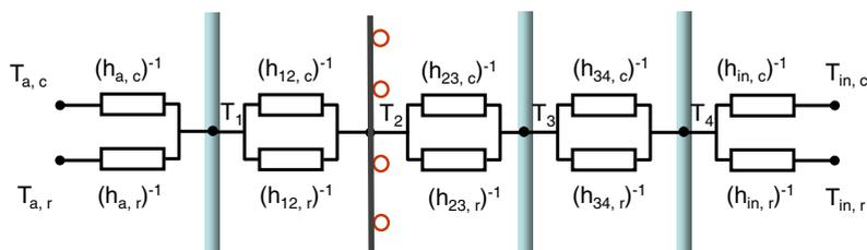
Fig. 2. Simplified, one-dimensional thermal resistance network of an insulating glass flat plate collector, referred to the undisturbed, “centre-of-glass” region of the panel
