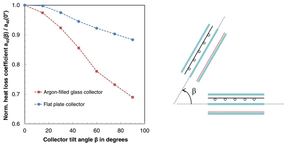
Fig. 4. Calculated normalized “center-of-glass” heat loss coefficient  $a_{40}(\beta)/a_{40}(0^\circ)$  in dependency of the tilt angle for an argon-filled, triple-glazed glass collector with a low-e inner pane compared to that of a common flat plate collector, as reported in [11]
