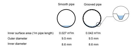
Fig. 5. Geometric shape and dimension of the grooved pipe compared to the smooth pipe as a reference, the condensate flow in the evaporator zone is schematically illustrated.
