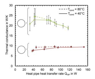
Fig. 6. Measured thermal conductance of butane filled heat pipes at condenser temperatures of  $T_{cond} = 40^{\circ}$ C and 80°C with smooth inner surface compared to a pipe with grooved inner surface, both with the same length of condenser and evaporator zone ( $l_{cond} = 260 \text{ mm}$ ,  $l_{evap} = 1730 \text{ mm}$ ).
