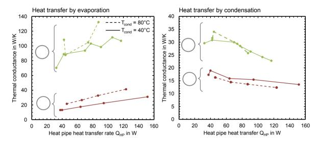
Fig. 7. Measured thermal conductances at the evaporator (left diagram) and the condensator (right diagram) of butane filled heat pipes at condenser temperatures of  $T_{cond} = 40^{\circ}$ C and 80°C with smooth inner surface compared to a pipe with grooved inner surface, both with the same length of condenser and evaporator zone ( $l_{cond} = 260 \text{ mm}$ ,  $l_{evam} = 1730 \text{ mm}$ ).
