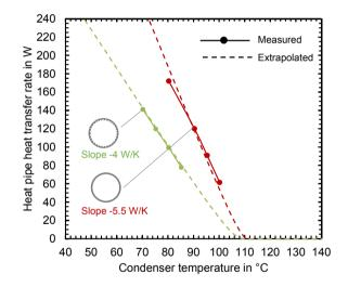
Fig. 8. Measured heat pipe heat transfer rate for varying condenser temperature in the range of the dry-out limit for with smooth inner surface compared to a pipe with grooved inner surface, both with the same length of condenser and evaporator zone (l<sub>cond</sub>= 260 mm, l<sub>evap</sub>= 1730 mm).
