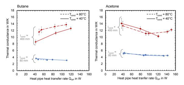
Fig. 3. Measured thermal conductance for butane-filled heat pipes (left diagram) and acetone filled heat pipes (right diagram) with different condenser lengths  $l_{cond} = 80$  mm and 400 mm for two different condenser temperatures ( $T_{cond} = 40^{\circ}$ C and  $80^{\circ}$ C)
