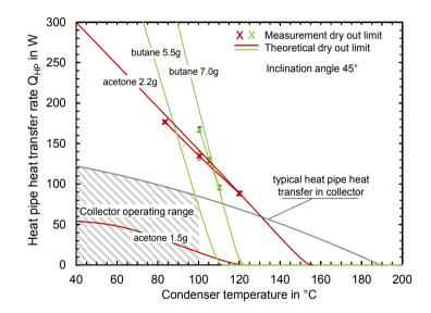
Fig. 4. Measured and calculated heat pipe heat transfer rate in the range of the dry out limit for butane (mass of 7.0 g and 5.5 g) and for acetone (m = 2.2 g and m = 1.5 g) compared to the typical heat transfer of one heat pipe in a solar collector.
