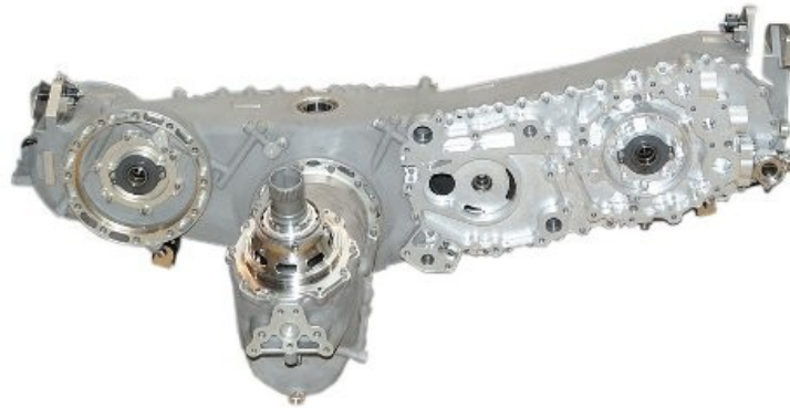
Figure 3 – Hispano-Suiza accessory gearbox and power transmissions for the Rolls-Royce's Trent family of engines powering the Airbus A340-500/600, Airbus A330, and Boeing 777. Visible are the connection for the radial drive shaft and the mounting pads for the accessories [16]
