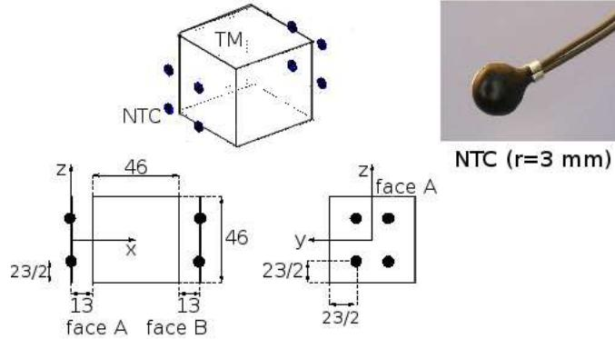
**Figure 1.** Situation of the thermistors surrounding the *TM*. Units in mm.
