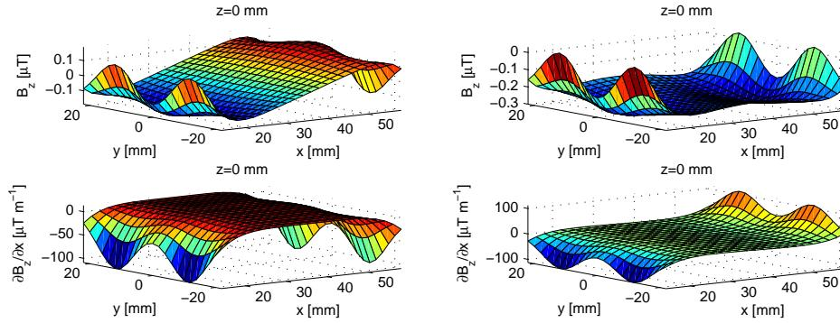
**Figure 4.** Representation of the  $z$ -component of the magnetic field and magnetic field gradient in the equatorial plane of TM. Left: Configuration A (see figure 3). Right: Configuration B (see figure 3).
