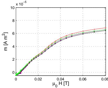
**Figure 5.** Measured *FMC* for a set of BetaTherm thermistors.
