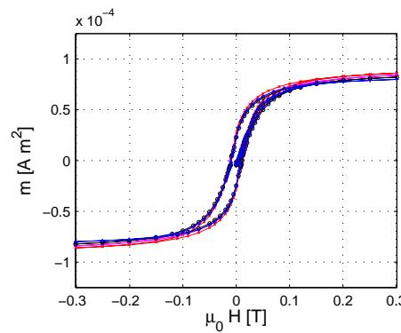
**Figure 2.** Hysteresis curve at 300 K for the set (four samples) of 10 kΩ NTC thermistors of BetaTherm.
