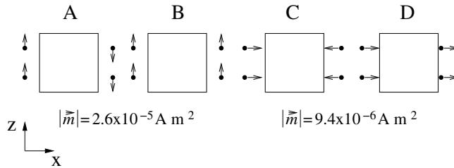
**Figure 3.** Configuration analysed for the magnetic field and magnetic field gradient calculations. This four configurations cover the worst cases involved in the problem. Intermediate configurations lead to smaller values of the magnetic field and magnetic field gradient in the TM. Arrows stand for the NTC's magnetic moment orientation [6].
