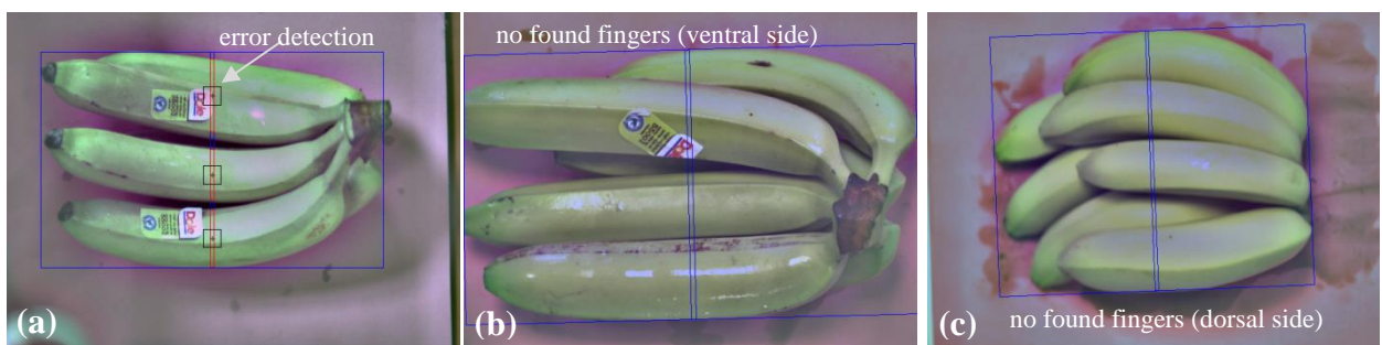
Fig. 5.17. False localization of the 2D codes on banana hands
