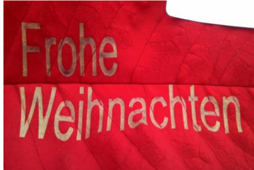
Fig. 5.22. Laser marking on poinsettia leaves using 0.5 W [0.55 J per character]
