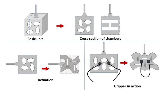
**Figure 4.** Vacuum-operated buckling FEA actuators, based on [51].
