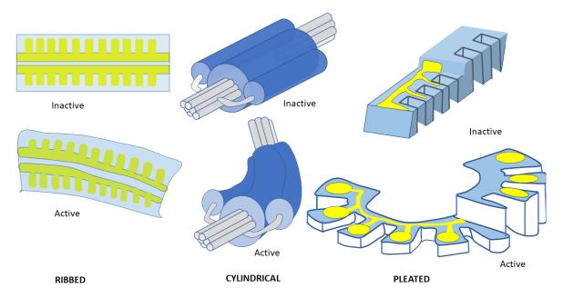
Figure 2. Ribbed, cylindrical, and pleated FEA, based on [7].
