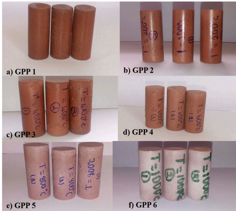
Figure 3. Photos of unheated and heated metakaolin-phosphate-based geopolymer cements. (a) GPP1, (b) GPP2, (c) GPP3, (d) GPP4, (e) GPP5 and (f) GPP6.
