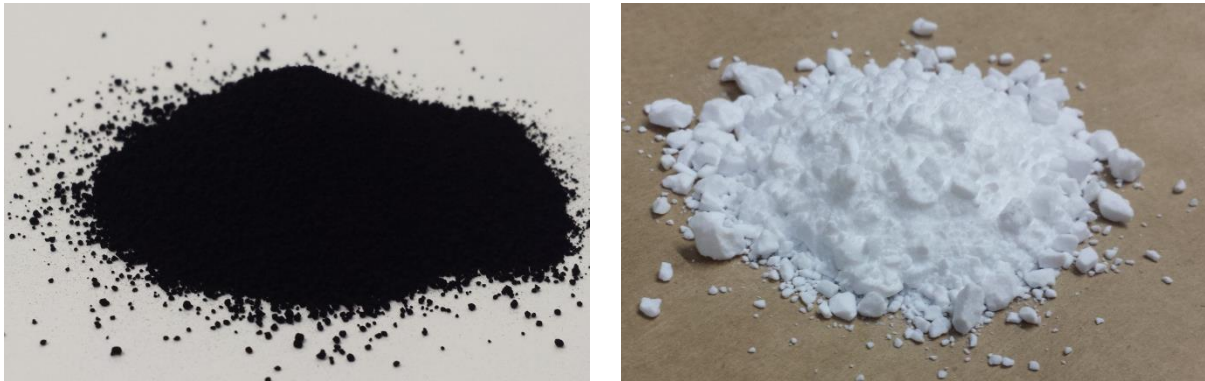
Figure 8: Reinforcing rubber fillers: carbon black on the left and silica on the right.
