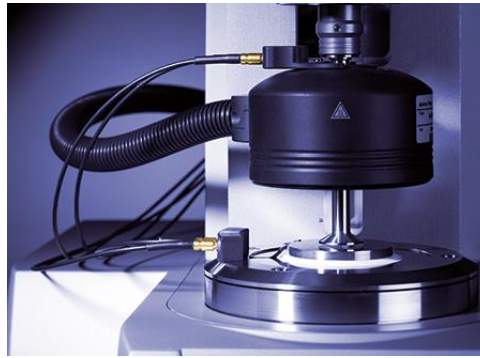
Figure 37: Setup for combined rheological and dielectric testing of elastomer composites [168]. The four thin cables connect the lower and upper plates of the measurement cell to dielectric spectrometer in order to create a dielectric closed loop.
