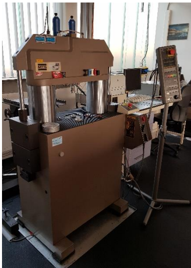
Figure 31: Multihysteresis measurements for fitting with the DFM. The dynamic mechanical analyser MTS is shown on the left. The measurement setup is depicted on the right.
