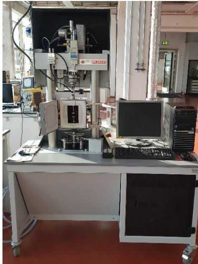
Figure 34: The dynamic mechanical analyser Eplexor ® 500 N is shown on the left. The measurement cell is shown on the right.
