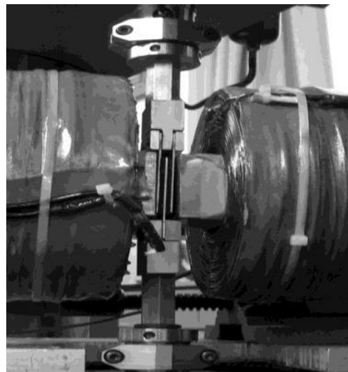
Figure 31: Multihysteresis measurements for fitting with the DFM. The dynamic mechanical analyser MTS is shown on the left. The measurement setup is depicted on the right.
