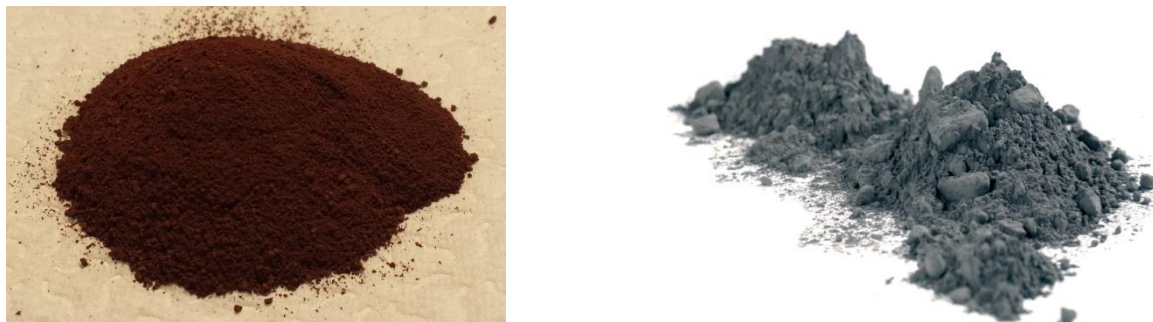
Figure 19: Magnetic fillers used. MAGSILICA is on the left. CIP is on the right [114].
