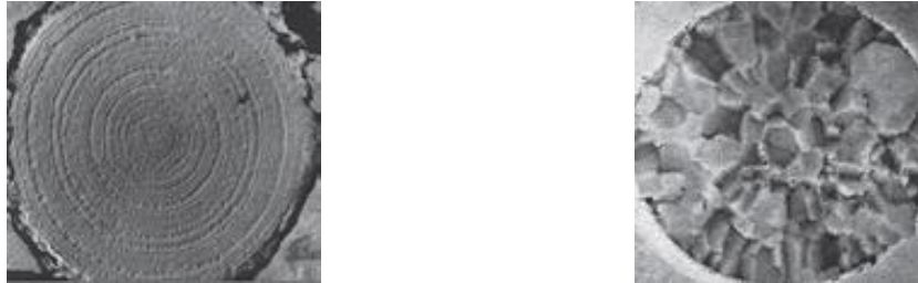
Figure 17: Structure of carbonyl iron particles. Onion skin structure of hard grade CIP is depicted on the left. The right picture illustrates the polycrystalline structure of soft grade CIP [114].
