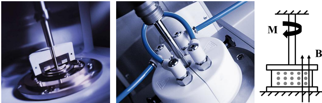
Figure 36: Setup for combined rheological and magnetic testing of elastomer composites. On the left, the device for rheological measurements is shown. Magnetic investigations occur in closed space shown in the middle picture in order to prevent magnetic losses [167]. On the right, the measuring principle is schematically drawn.
