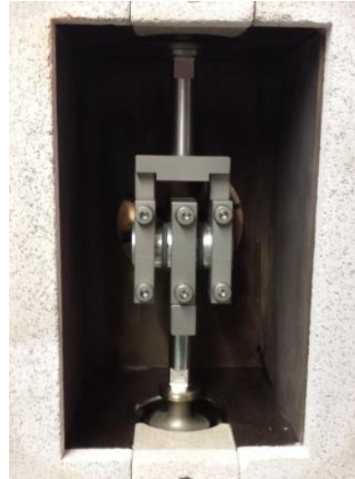
Figure 34: The dynamic mechanical analyser Eplexor ® 500 N is shown on the left. The measurement cell is shown on the right.
