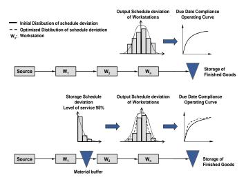
Fig. 3 The results of a better schedule adherence within the storage for finished goods
