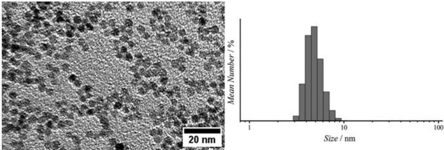
**Figure 1.** The transmission electron micrograph reveals a particle size of 5 nm (left). Dynamic light scattering measurements show a narrow size distribution with a mean value of 5 nm (right).
