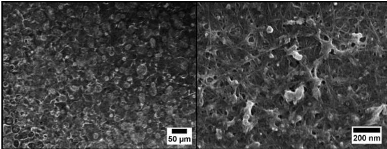
**Figure 3.** Microscopic investigations of the SWNT layer. Left: Light microscope image, showing circle-shaped structures, caused by the spraying process. Right: SEM image showing dense network of intertwined nanotubes.
