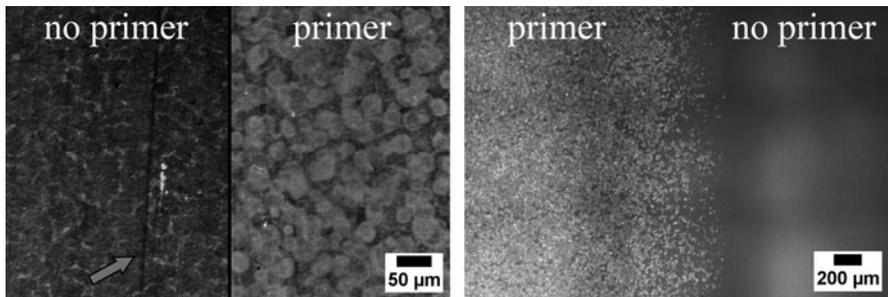
**Figure 5.** Light microscope images of the films after scratching tests (left) and after wiping tests using a wet cotton swab (right).
