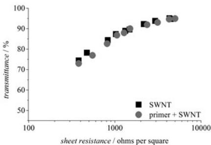
**Figure 4.** Samples with a primer layer show the same performance with regard to sheet resistance and transmittance as the samples prepared without priming.
