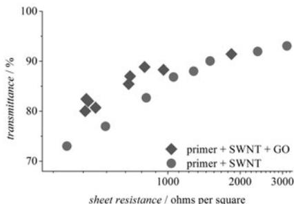
**Figure 6.** Samples with a top layer of graphene oxide show a better performance than those without such a layer, i.e. at a certain transmittance their sheet resistance is smaller or at a certain sheet resistance their transmittance is higher.
