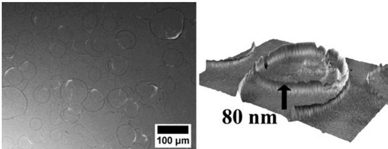
**Figure 2.** Confocal microscopy of zinc oxide primer layer. Left: Bright field image of zinc oxide nanoparticle agglomerations on the substrate. Right: Stacked confocal images with height informations.
