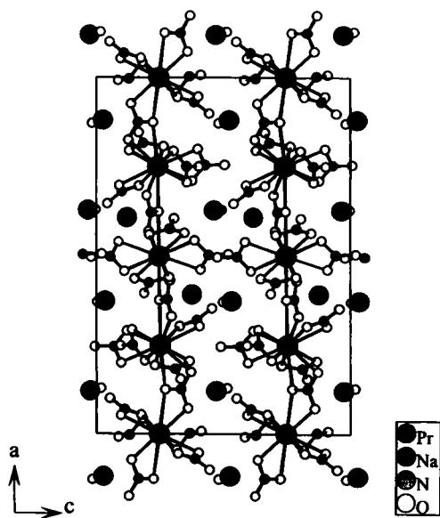
Source of material:  $\text{Na}_2[\text{Pr}(\text{NO}_3)_5] \cdot \text{H}_2\text{O}$  crystallizes from a solution of  $\text{Pr}_6\text{O}_{11}$  and  $\text{NaNO}_3$  in conc.  $\text{HNO}_3$  upon slow evaporation in a desiccator over solid KOH. It is also obtained from a solution of  $\text{Na}_3\text{Nd}_2(\text{NO}_3)_9$  in acetonitrile by isothermal evaporation in a slow stream of argon.
