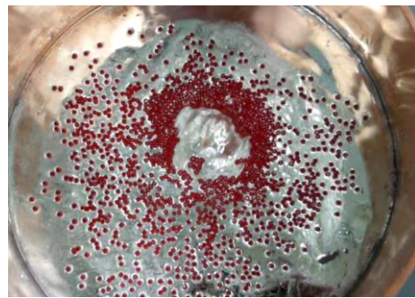
Fig. 13: Particle “slag” distribution; h_0=20\text{mm} , I_{\text{rms}}=1000\text{A}
