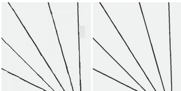
Fig. 9. Predicted signals for a synthetic example: it is observable that CoMIC (left) and HEVC (right) can generate a similar prediction for linear structures.
