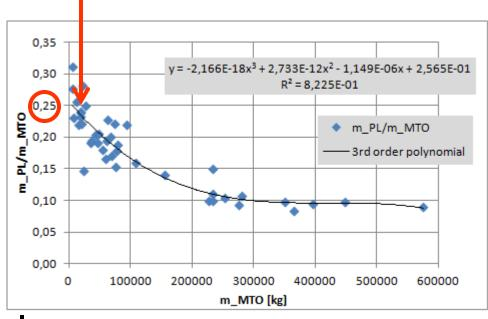
Payload, m\_PL calculated from "typical number of seats" from manufacturers seat layout and 93 kg/seat. Data points represent passenger aircraft most frequently in use with 19 seats or more. Note: Although the regression is quite good, physically m\_PL/m\_MTO is a function of range.
