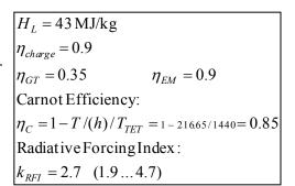
Due to flight at altitude plus energy mix with renewables & nuclear power:  $m_{CO2,eq,kerosene} \approx 2.5 \cdot m_{CO2,eq,battery}$
