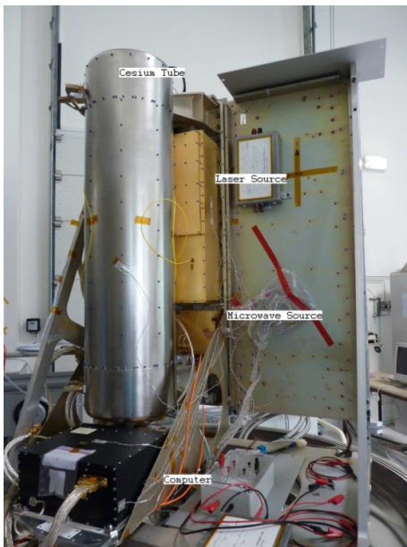
Figure 5.10.: The PHARAO engineering model under test. The Pharao Cesium tube is approximately 1 m in length. [52]
