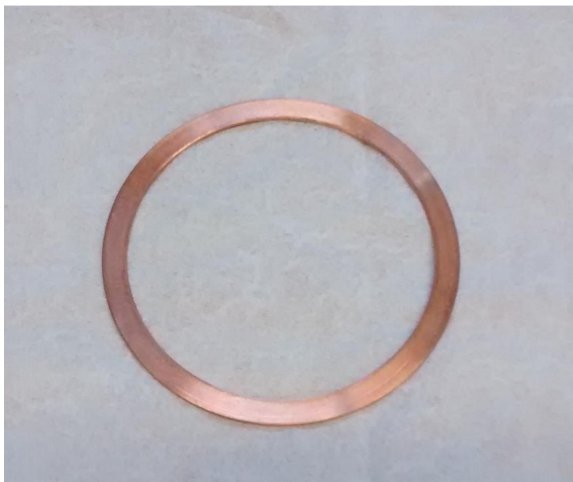
Figure S2: This photograph displays a copper spacer with a thickness of 0.8 mm. The spacer enhances the intensities by increasing the distance between the sample cone and the skimmer cone.
