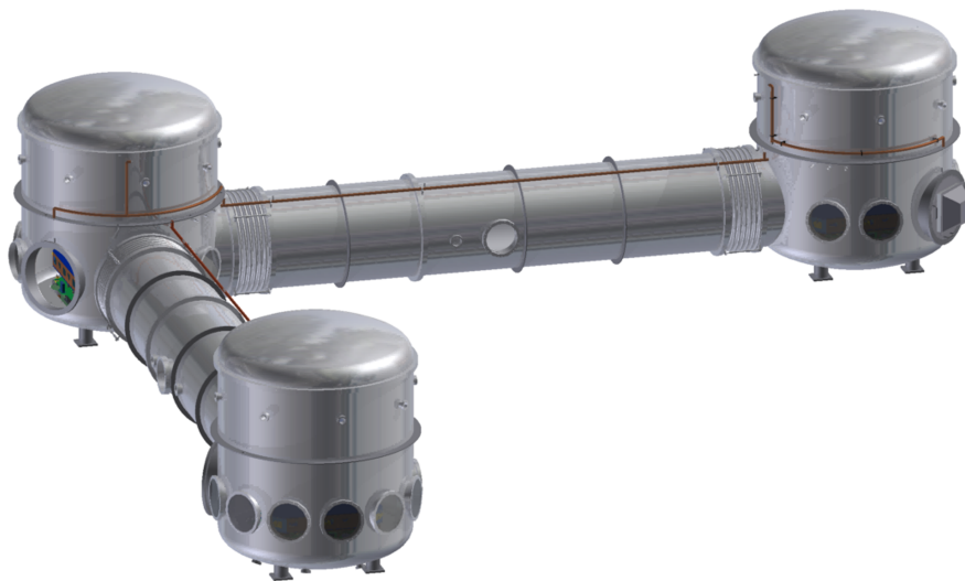
Figure 2.1: Rendered image of the vacuum system of the AEI 10 m Prototype. The vacuum system is L-shaped and consists of three vacuum tanks. They are connected via vacuum tubes and separated by 10 m. Three seismically isolated optical tables are placed inside the tanks. Picture courtesy of G. Bergmann
