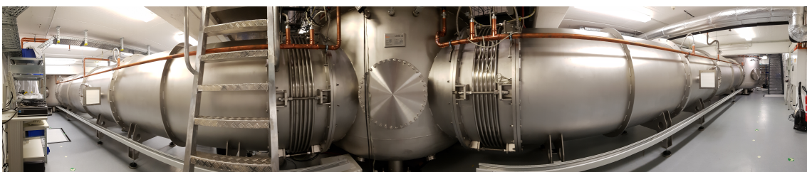
Figure 2.4: Vacuum system for the AEI 10 m Prototype Interferometer consisting of three tanks connected via steel tubes. The system encloses a volume of 100 \text{ m}^3 . Each tank has a diameter of 3 m and a height of 3.4 m and hence allows in-vacuum installation and commissioning work. Inside each vacuum tank three seismic isolated tables are placed to isolate the components such as optics from ground motion. The table centers are separated by 11.65 m. Several pumps allow a fast pump down of the system. A pressure of 10^{-6} ha Pa can be reached within some hours while further pumping leads to a pressure of 10^{-7} ha Pa after one week. Picture courtesy of P. Oppermann.
