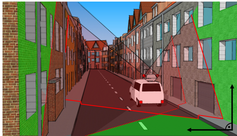
Figure 13. Exemplary illustration of a scenario for information-based georeferencing of a kinematic MSS (white vehicle) with classified building facades and road surface (green), as well as their geometric relation (black).
