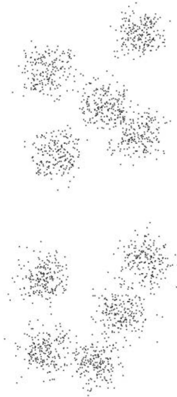
Fig. 3. Two snapshots of transceiver positions in the ECRM mobility model. The upper panel is at time zero (after a 200 second run to remove the effects of initial positions), and the lower panel is 900 seconds later. Because of the grouping nature of the model, there is a noticeable difference in the distribution of positions with respect to time.
