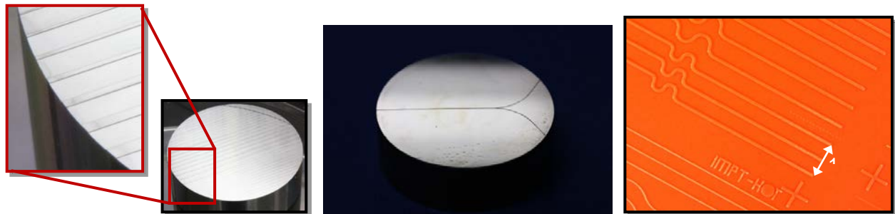
Figure 4. Left and middle: master tools realized by precision milling containing straight rib-structures in aluminum and bent trench structures in tin, respectively. Right: Rib-structures on a silicone embossing stamp, see [13].
