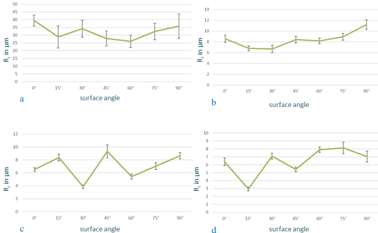
Figure 6: Surface roughness of the different facets of the sample for three initial situations and their standard deviation; a) reference samples as printed, b) honed, grinded and polished without pretreatment, c) honed, grinded and polished with sand blasting as pretreatment and d) grinded and polished with ball cutting as pretreatment
