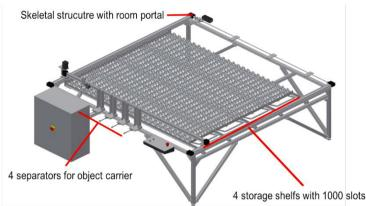
Figure 4: Construction of the sorting system
