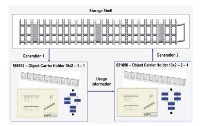
Figure5: New Generation according to Technical Inheritance for the object carrier holder
